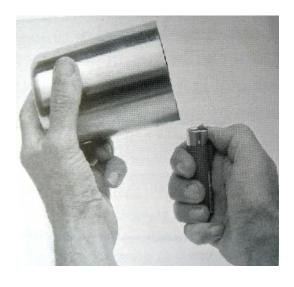
2) Carefully ignite the methanol in the sample cup. Allow the methanol to burn for several seconds.
