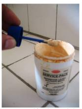
3) If you want to verify the weigh, put those 8 spoons of Lauryl Sulphate powder on a piece of paper. Switch on the balance and weigh to verify the amount of Lauryl Sulphate. Pour the Lauryl Sulphate in the metal cup into the 50ml of water. Shake it gently to dissolve the powder.
