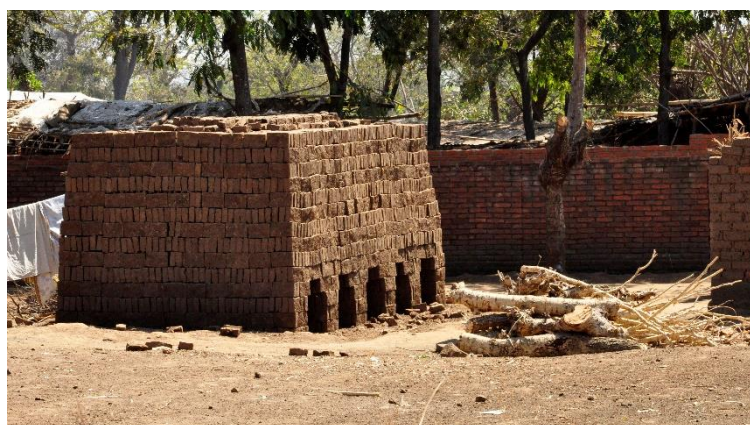
Figure 3 – Oven for bricks and firewood. Abadia (2016)
