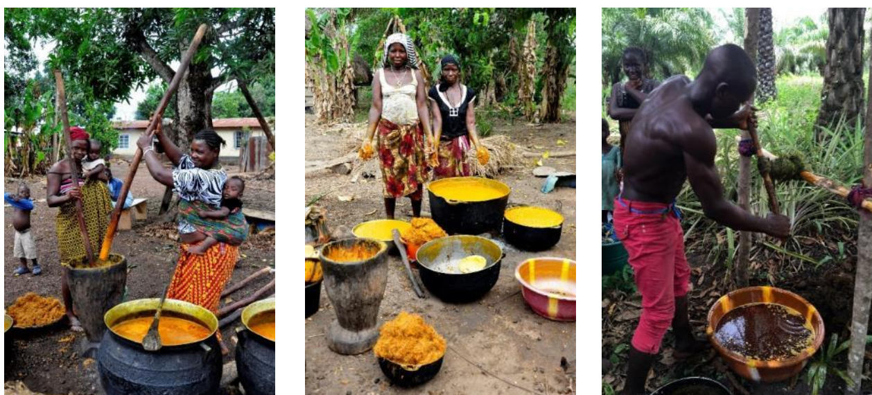
Figure 15 - Traditional palm oil processing steps. Abadia (2017) (from left to right: crushing within a mortar; washing of fibres; squeezing with a local rope press).
