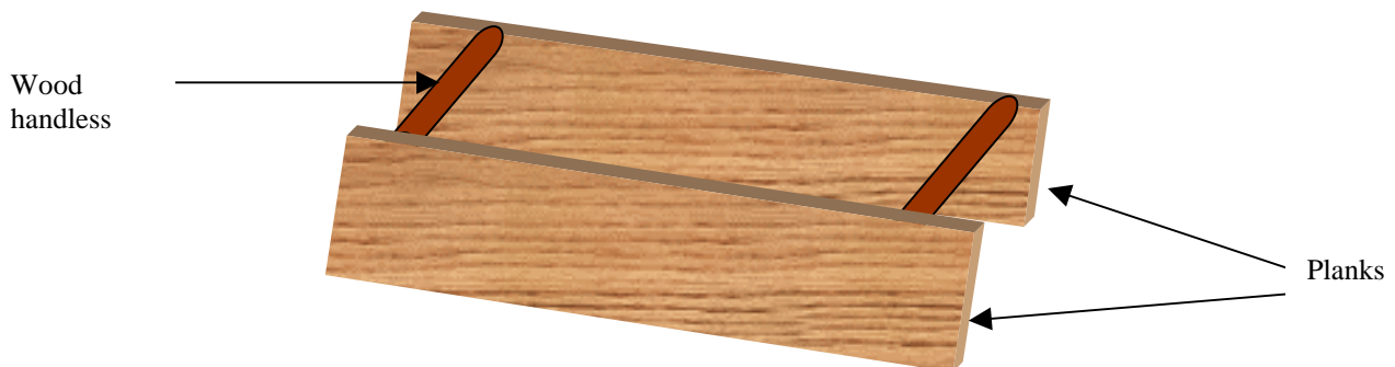
Fig. 6 : Crib for laying gravel
