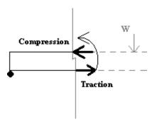
Let's consider now the section of the beam. Appear on it a moment M and practically on this section this moment could be describe by to yield: a traction and a compression.
