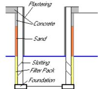
base of the well and the mortared brick work is built up to 300 mm above the ground level. If possible,
