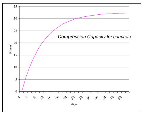
commonly use a Cement 30. It means the concrete could resist to 30 N/mm² after 28 days (See Compressive Test).
