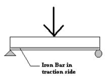
One of the characteristics of concrete is its poor resistance to traction.
