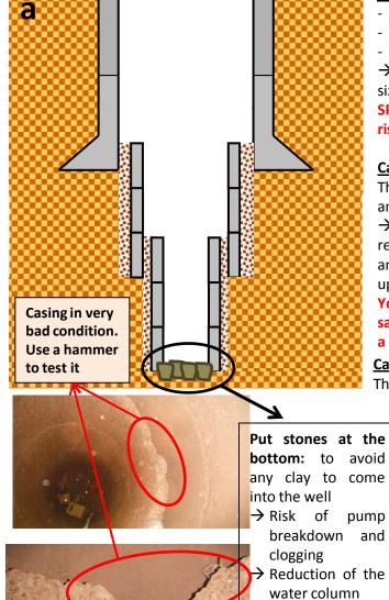
The original casing is in very bad condition: it cannot support a new construction
