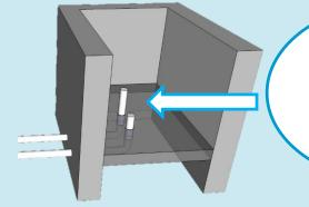
Removable overflow pipe serve as simple and robust washout for easy cleaning operations
