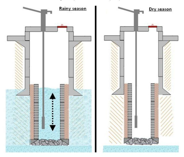
This situation usually happens when a well construction is not properly planned, designed and constructed. Timing the sinking of a well to correspond to low aquifer levels belongs however to standard practices (especially in the absence of a dewatering pump). Poorly designed and underdeveloped wells are then also subject to more frequent pump failures.
