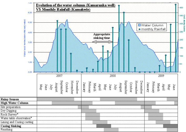
\*Rock Survey to drill the bottom of the well with rods in order to assess the presence of stone
