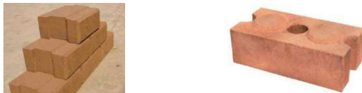
Figure 7: Two classic interlocking blocks made using a SSB press. On the right a model of an interlocking block with a site for an iron bar passing inside. The both shape are designed to use zero/little quantity of mortar.
