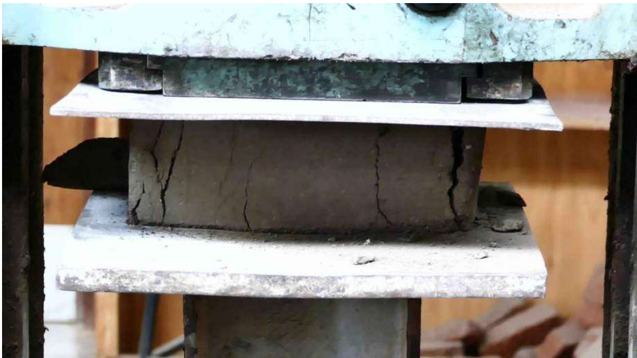
Figure 24: compression test on a SSB block taken in a targeted village at the final breaking phase. The breaking point shown in this picture is at 2.2 N/mm 2 .
