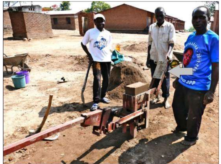
Figure 13: the SSB press in the open position. The block is completely out, ready to be hold and put outside the mould
