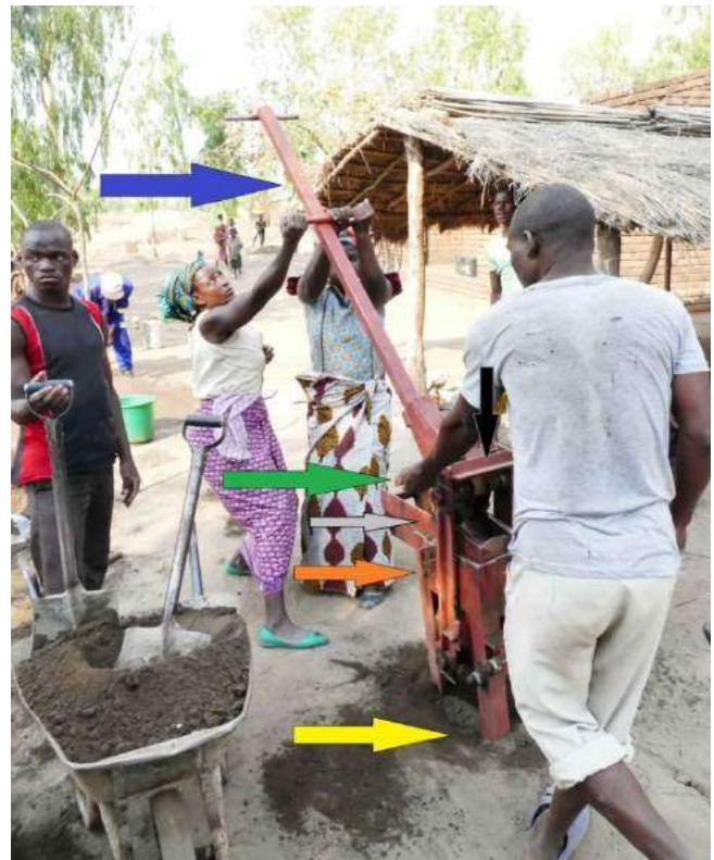
Figure 11: an SSB press in a pressing phase. Blue arrow: the press handle is in correctly positioned in a diagonal position, not too vertical and not too horizontal, indicating that the amount of soil mixture in the mould is correct; Black arrow: upper lock of the plate. Green arrow: the volunteer is correctly accompanying the press handle system using the side handle by the left hand; Grey arrow: closing plate of the mould; Orange arrow: the 2 plates that should be tied by a wire during transport and non-working time; Yellow arrow: the press machine feet are dug in 30/40 cm below the ground level.
