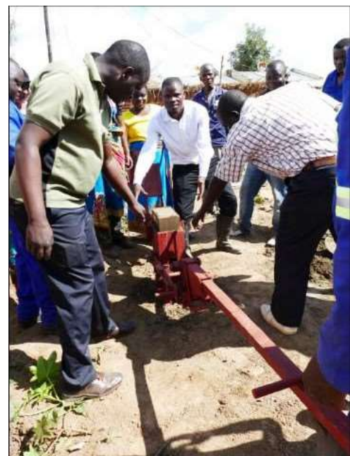
Figure 6: Phalombe WASH team is testing the use of the SSB press for the first time.
